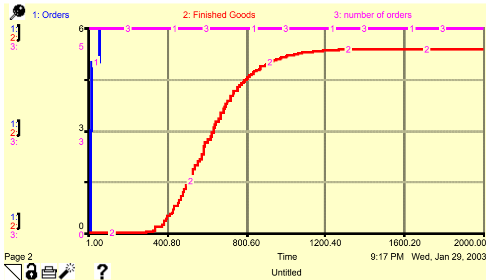
Figure 12, Graph of Time to Produce 5 units of Finished Goods with TOC in place
